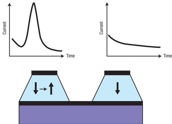
**Figure 2** The electric dipoles in the ferroelectric layers (pale blue) of the nanocapacitors built by Lee *et al.* can point up or down, and can be switched by applying a voltage of the correct polarity to the upper electrode (left). When this happens, a distinct peak is measured in the current through the device. However, when the dipole is already aligned with the applied voltage, the current does not contain any distinctive features (right).
