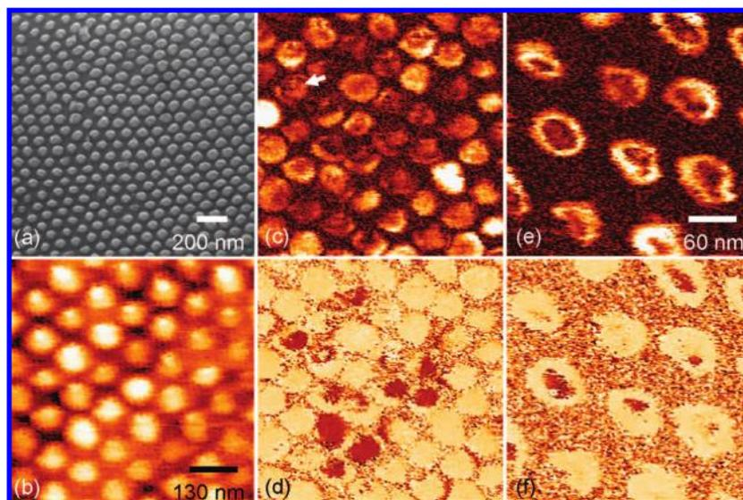
**Figure 1.** (a) SEM and (b) topography images of PZT (40/60) nanodot arrays. (c, d) VPFM amplitude and phase of the nanodot arrays shown in (b). (e, f) Higher resolution VPFM amplitude and phase images from another location within the nanodot array. The scale bar in (b) refers to (c) and (d), while the scale bar in (e) refers also to (f). The vertical data range in (b) is 18 nm.
