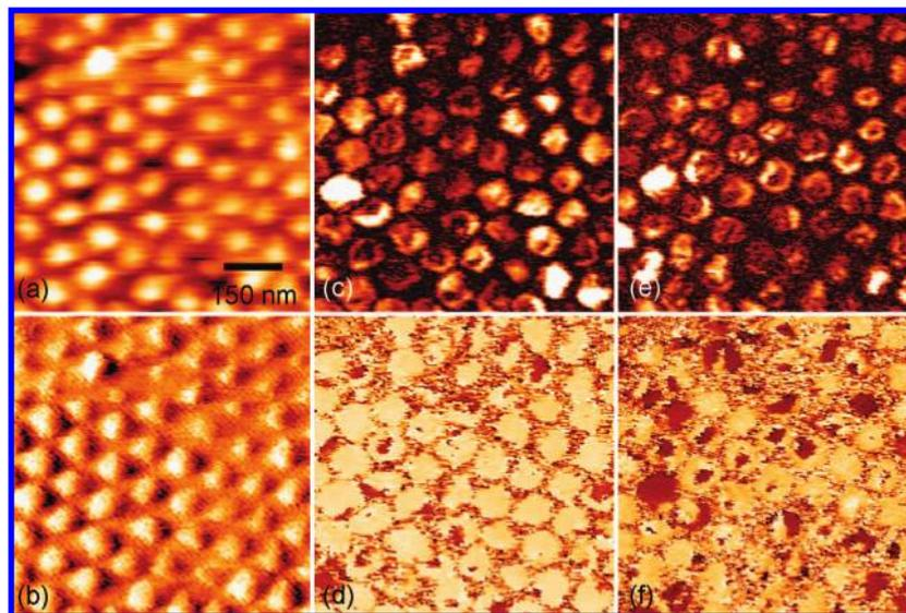
**Figure 2.** (a) Topography and (b) error signal images of a PZT (40/60) nanodot array. (c, d) VPFM and (e, f) LPFM amplitude and phase images from the location shown in (a, b). The scale bar in (a) refers to (b–f) as well. The vertical data range in (a) is 20 nm.
