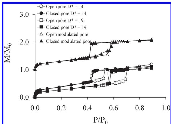
**Figure 4.** Simulated Ar adsorption isotherms at 85 K in regular and modulated AAO pores, opened at both ends and closed at one end. The curves for the modulated pores have been shifted up by +1 for the sake of clarity.
