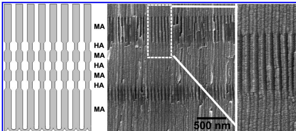
**Figure 1.** (left) Schematic diagram of a closed bottom modulated pore with  $N = 3$ . (right) Cross-section micrograph of the AAO membrane showing the modulations in pore diameter and an enlarged view of them.
