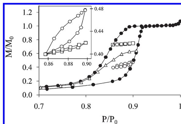
**Figure 3.** Experimental capillary condensation hysteresis loop for Ar in closed bottom pores with three modulations. A primary descending scanning curve and two subloops are also shown. The inset shows a comparison of the two subloops.
