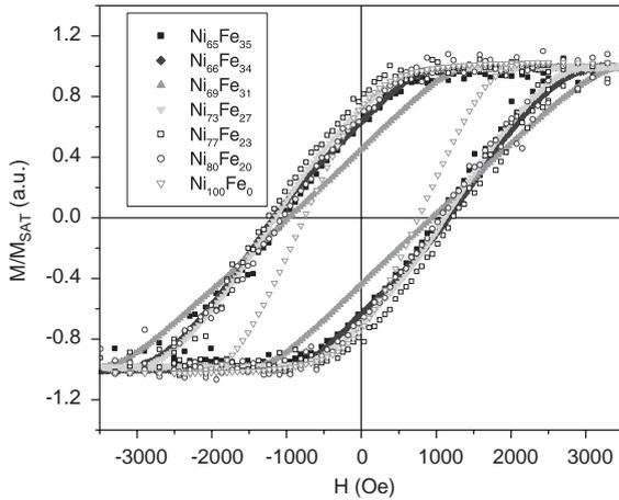
Fig. 3. Axial hysteresis loops of NiFe nanowires arrays with different compositions.
