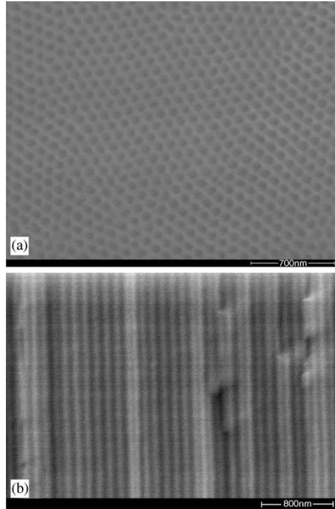
Fig. 1. SEM images of the (a) surface and (b) cross-section of a nanoporous alumina membrane.
