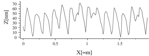
Fig. 4. The AFM image of  $\text{Ni}_{69}\text{Fe}_{31}$  array of nanowires, and filling profile along an indicated orientation.
