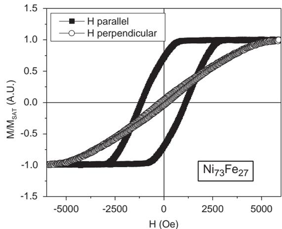
Fig. 2. Hysteresis loops of a  $\text{Ni}_{73}\text{Fe}_{27}$  filled alumina membrane measured with applied field parallel (■) and perpendicular (○) to the nanowires axis.
