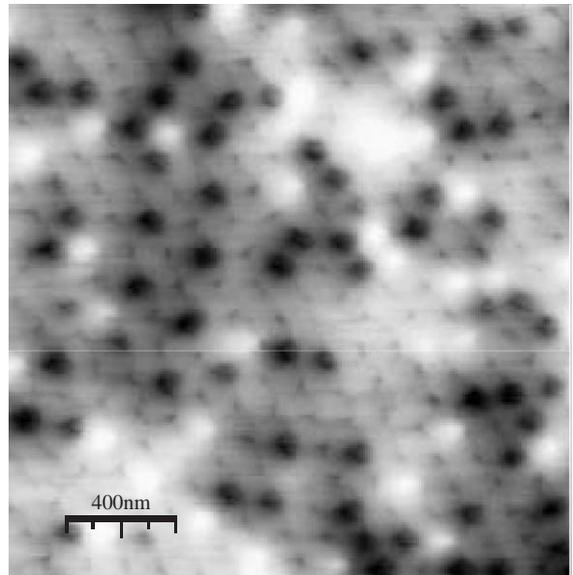
Fig. 5. An MFM image of  $\text{Ni}_{69}\text{Fe}_{31}$  array of nanowires.
