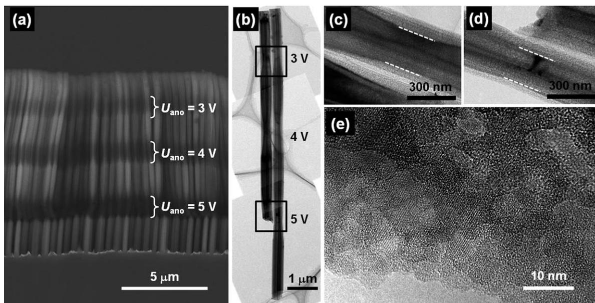
**Fig. 2** (a) SEM image of [100] SiNWs prepared by pulsing of anodic bias during metal-assisted chemical etching of Si(100) wafer, showing the effect of pulse amplitude ( $U_{\text{ano}}$ ). (b) TEM micrograph of SiNWs taken from the sample shown in panel a. (c and d) Magnified TEM images of the porous segments formed at  $U_{\text{ano}} = 3$  V and  $U_{\text{ano}} = 5$  V, respectively. (e) High-resolution TEM image, showing the morphology of porous segment.
