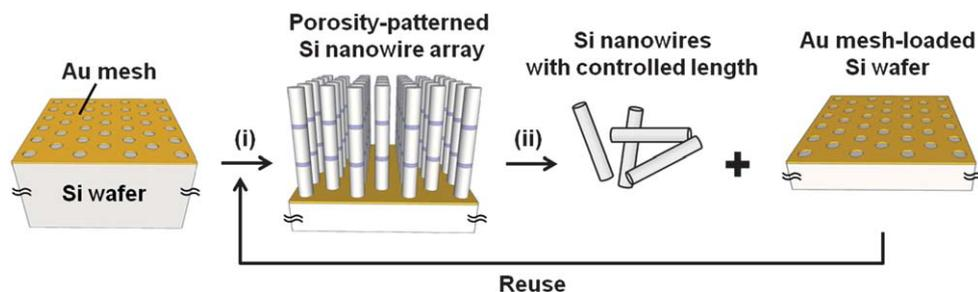
**Scheme 1** Schematic diagram of the continued mass fabrication of SiNWs with prescribed lengths by (i) periodic pulsing of anodic bias during metal-assisted chemical etching of a silicon wafer and subsequent (ii) ultrasonic treatment of the resulting porosity-patterned SiNWs. The remaining gold mesh-loaded silicon wafer can be used again for the preparation of SiNWs with desired lengths.
