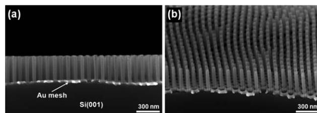
Fig. 4 Representative SEM images of SiNW arrays fabricated by MaCE of the Si(001) substrate in a mixture solution of HF and  $\text{H}_2\text{O}_2$  [HF :  $\text{H}_2\text{O}_2 = 2 : 1$  in v/v]: (a) cross-sectional view and (b) tilt-view.
