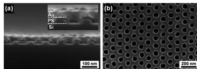
Fig. 5 SEM images of patterned PS (40 nm) by  $\text{O}_2$ -RIE through an Au mesh mask: (a) cross-sectional view and magnified image (inset) without removal of the Au mesh and (b) top-view after removing the Au mesh using aqua regia.
