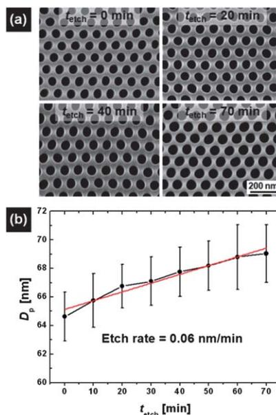
**Fig. 3** (a) Representative SEM images of the bottom side of the through-hole AAO membrane which was etched in 60 wt%  $HNO_3$  for varied etching times ( $t_{etch}$ ) for 0, 20, 40, and 70 min at room temperature (RT) and (b) variation of pore diameter ( $D_p$ ) as a function of  $t_{etch}$  and the linear fit (red trace).
