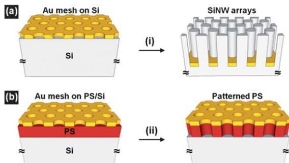
**Scheme 1** Schematics for the fabrication of (a) SiNW arrays via metal-assisted chemical etching (MaCE) of Si by utilizing the Au mesh as an etching catalyst and (b) patterning of the polystyrene (PS) layer through reactive-ion etching (RIE) of PS by employing the Au mesh as an etching mask, respectively.
