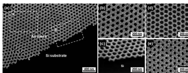
**Fig. 2** SEM images of an Au nanomesh transferred onto Si(001) wafer: (a) top-view at the edge of the Au mesh, (b) magnified view of the area denoted as A in (a) and (c) 45°-tilt-view of the squared area denoted as B, (d) top-view of the Au mesh replicated from 30-times reused AAO, and (e) top-view of the Au mesh with hole arrays of 48.2 nm in diameter.
