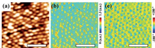
**Fig. 3** (a) Topography, (b) BE-PFM amplitude and (c) BE-PFM phase images of the PTO nanoislands in sample A. The BE-PFM images were obtained after topography measurements. Scale bars are 200 nm.
