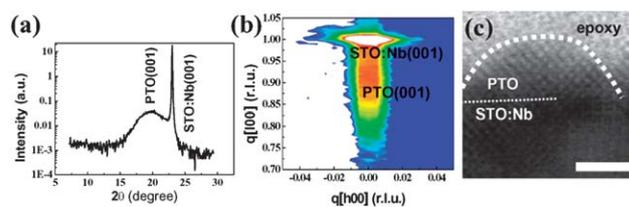
**Fig. 2** (a)  $\theta$ – $2\theta$  scan of sample B. (b) Reciprocal lattice space mapping around STO(001) in the HL-plane. (c) Cross-sectional TEM image of sample C. Scale bar is 2 nm.
