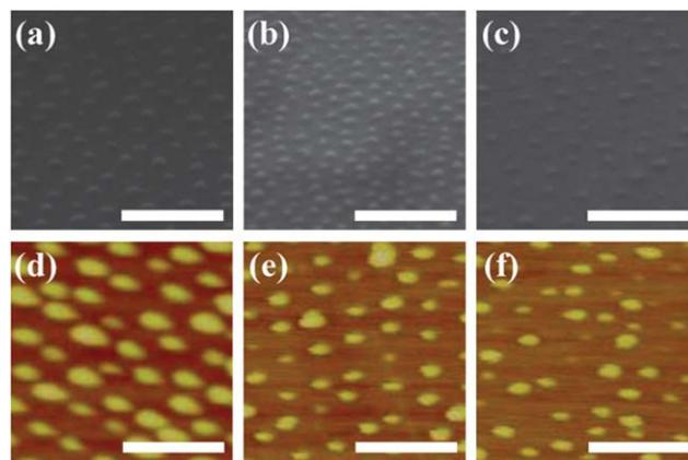
**Fig. 1** (top panels) SEM and (bottom panels) topography images of the three different PTO nanoisland arrays. (a and d) The left, (b and e) middle, and (c and f) bottom panels correspond to samples A, B, and C, respectively. Scale bars are 100 nm.
