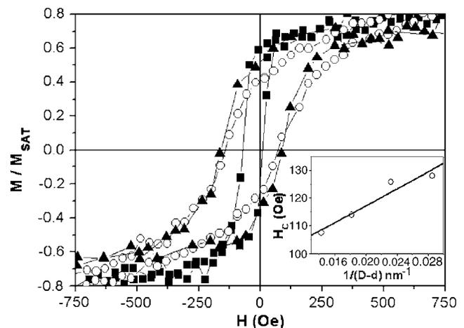
FIG. 4. In-plane loops for continuous film (■) and for two Ni nanoholes arrays [ $d=35$  (○) and 62 nm (▲) hole diameters]. Linear evolution of coercivity  $H_c$  with  $1/(D-d)$  ( $D$ =interhole distance) (Inset).
