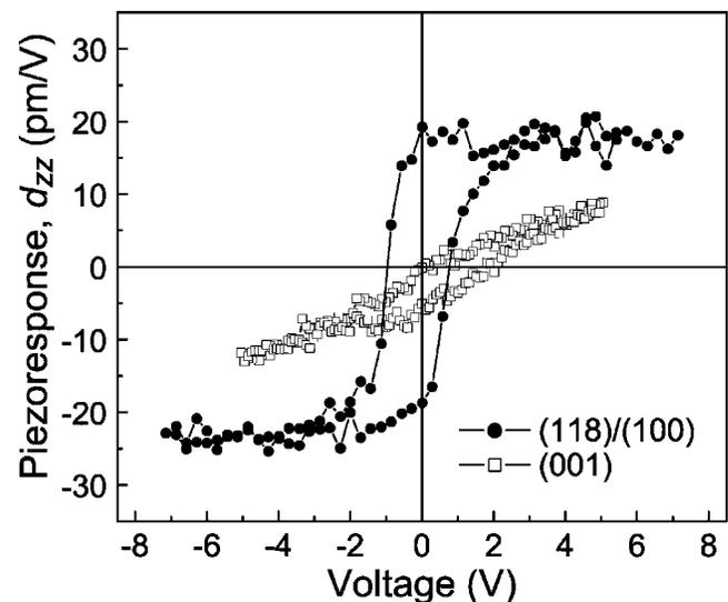
FIG. 4. Piezoelectric hysteresis loops of epitaxial BLT nanostructures with *c*-axis and non-*c*-axis orientation on (001)- and (011)-oriented SrRuO<sub>3</sub>/SrTiO<sub>3</sub> substrates, respectively.
