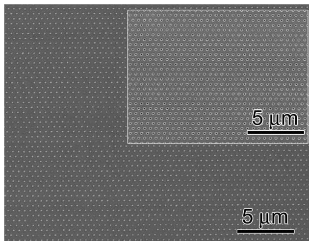
FIG. 1. SEM plan-view image of an as-deposited BLT nanostructure array on a  $\text{SrRuO}_3$  electrode on a  $\text{SrTiO}_3$  single-crystal substrate. The inset shows a SEM image of part of a gold nanotube membrane used for patterning.
