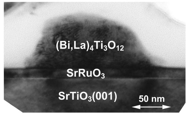
FIG. 3. TEM cross-sectional image of a crystallized BLT nanostructure on SrRuO<sub>3</sub>(001)/SrTiO<sub>3</sub>(001).
