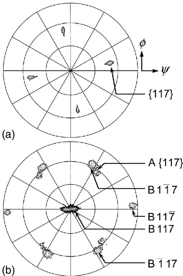
FIG. 2. XRD pole figures of (a) (001)-oriented and (b) (118)/(100)-oriented BLT nanostructure arrays epitaxially grown on SrRuO<sub>3</sub>-covered (001)- and (011)-oriented SrTiO<sub>3</sub> substrates, respectively. The fixed  $2\theta$  angle was  $30.1^\circ$  corresponding to the BLT 117 reflection. In (b), peaks originating from the (100)- and (118)-oriented parts of the BLT nanostructures are denoted “A” and “B”, respectively.
